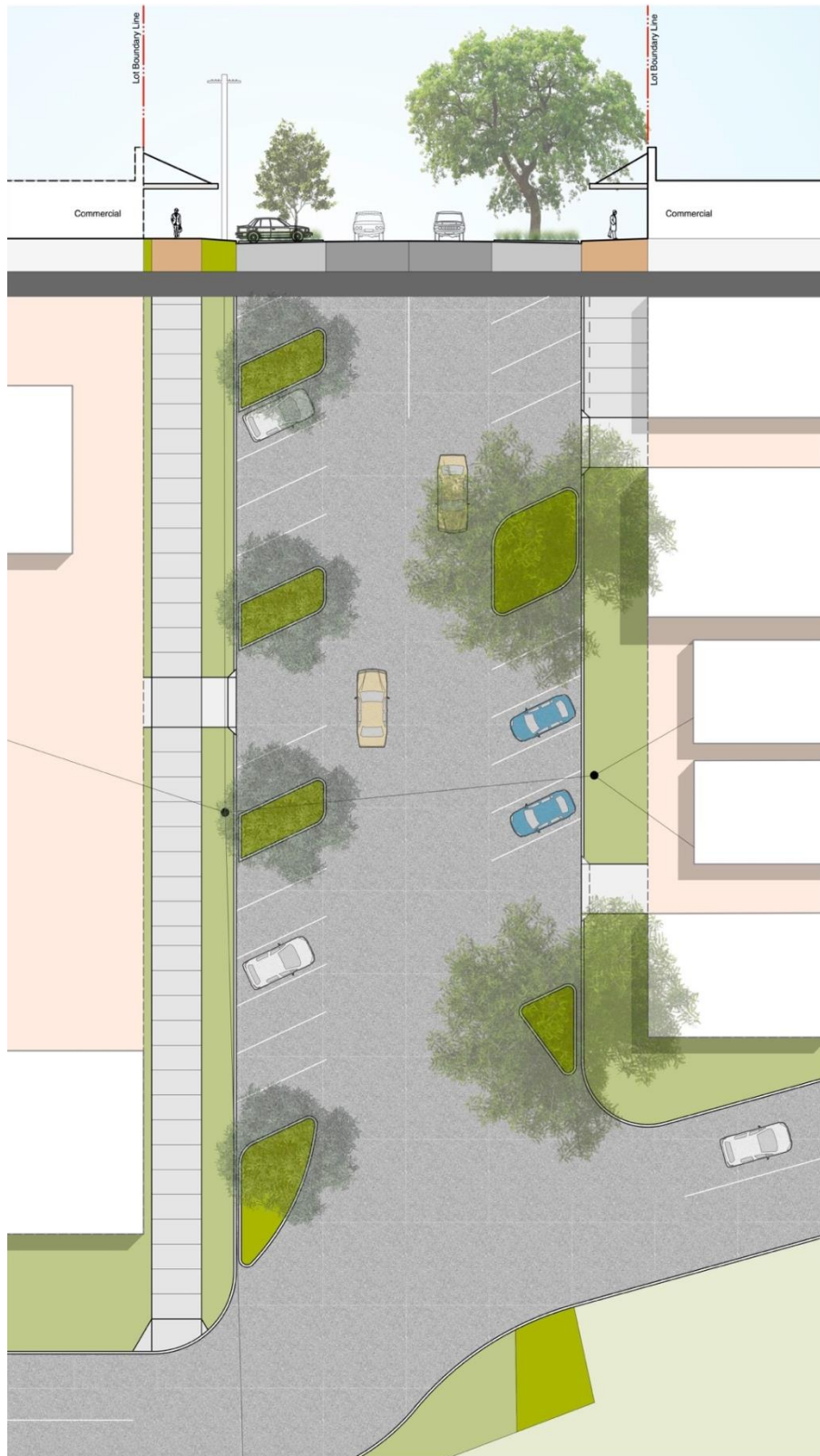
Figure 18: Typical treatment to Station Street between Cessnock Road & First Street
