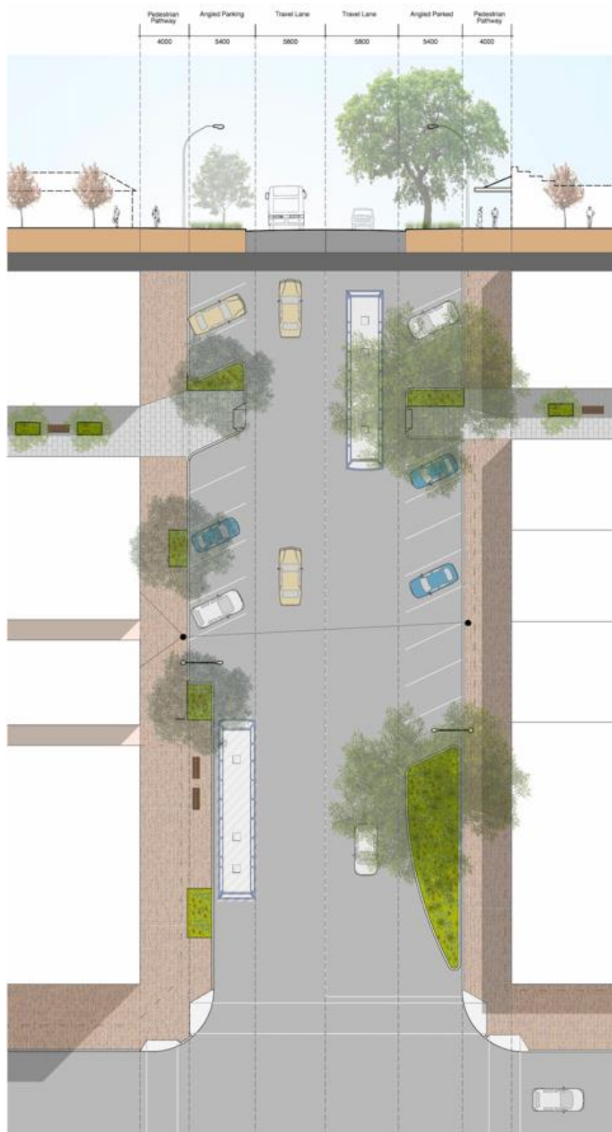
Figure 17: Typical treatment to Station Street between Cessnock Road & First Street
