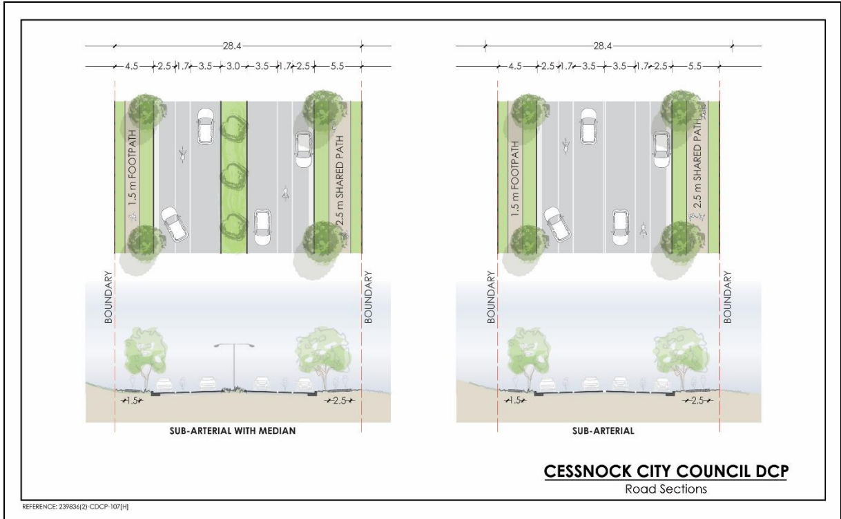
Figure 9: Road sections: Sub-arterial.
