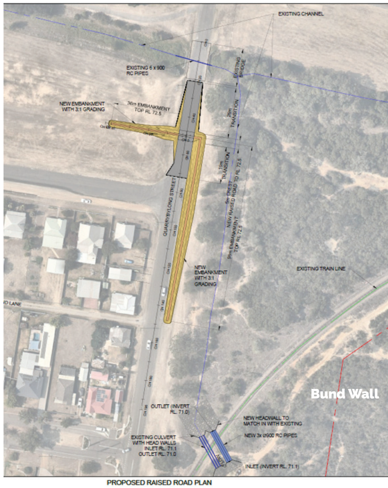
FIGURE 6 - RAISING OF QUARRYBYLONG STREET
