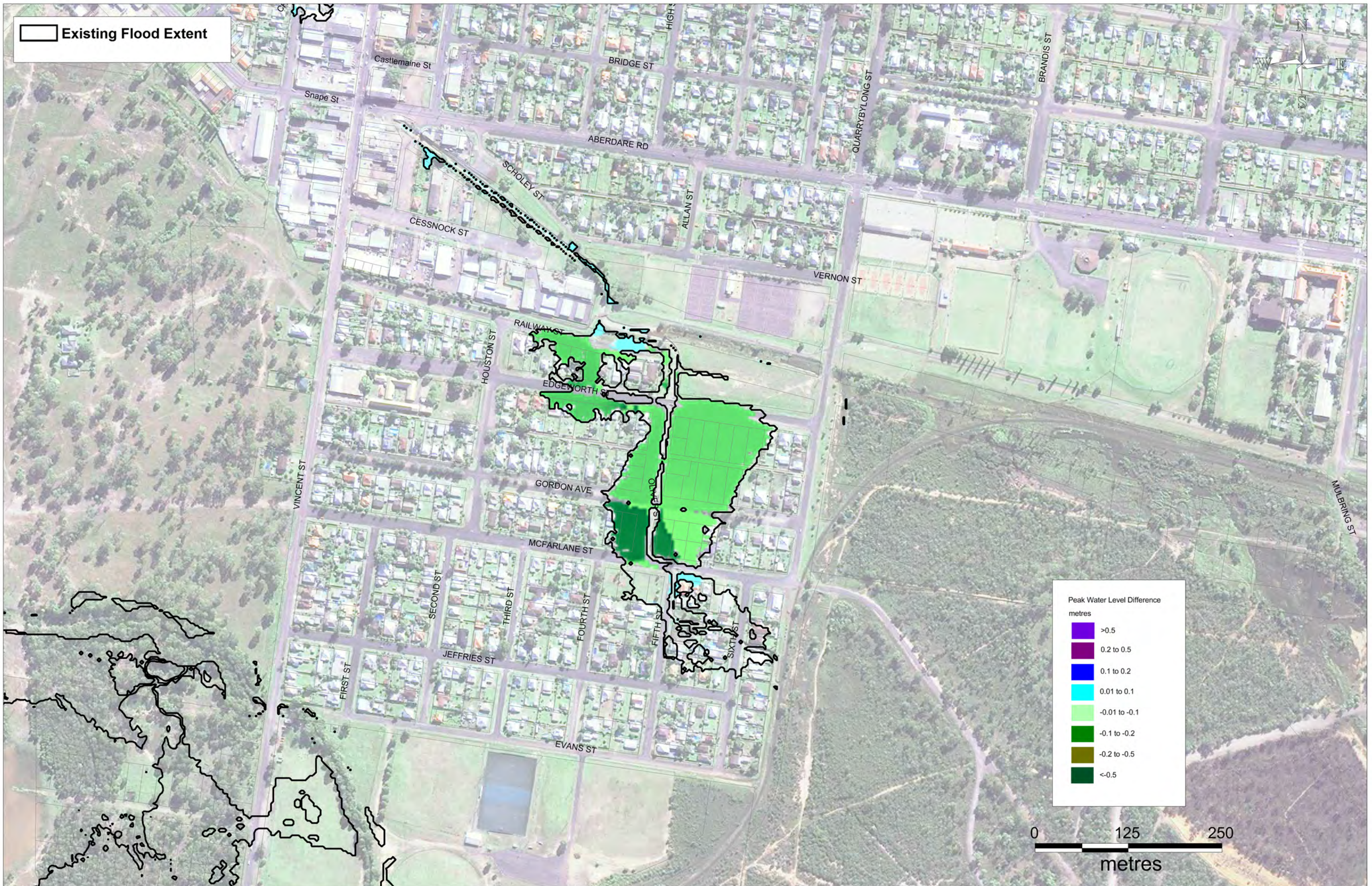
FIGURE 11-27 : APRIL 2015 STORM - PEAK WATER LEVEL DIFFERENCES FM4 Results Less Existing Results
