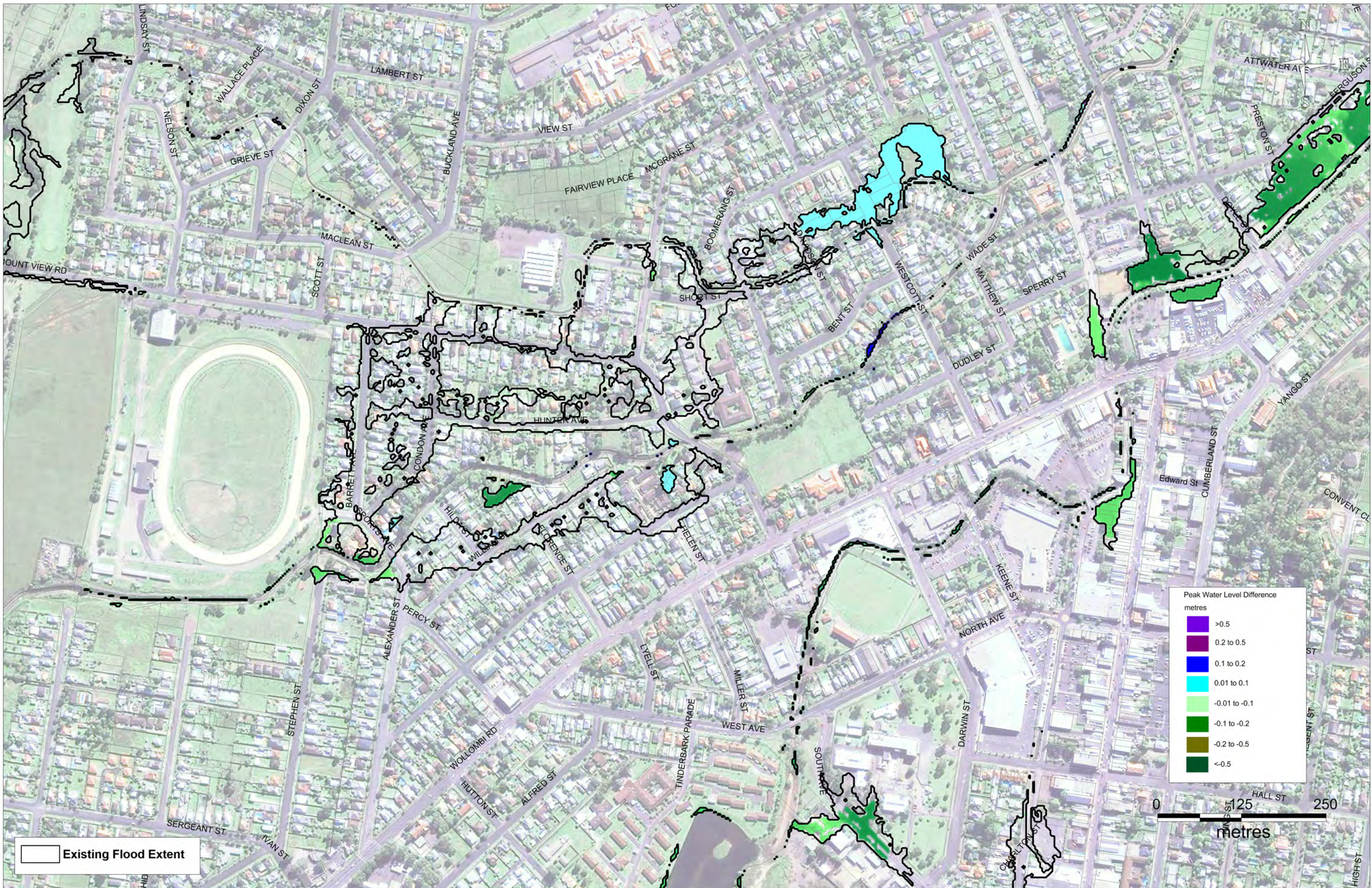
FIGURE 11-8 : 20% AEP - PEAK WATER LEVEL DIFFERENCES FM2 Results Less Existing Results
