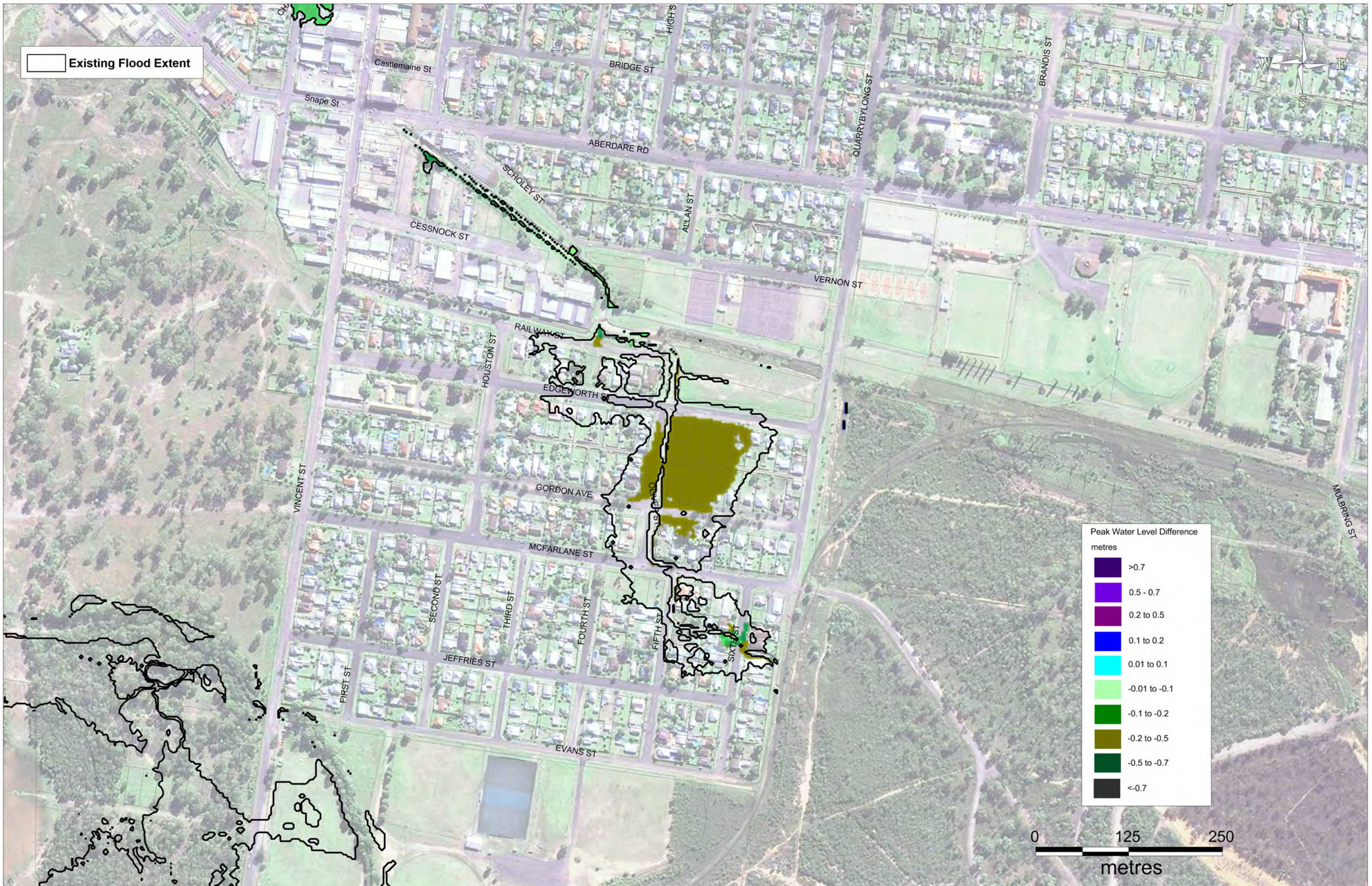
FIGURE 11-34 : APRIL 2015 EVENT- PEAK WATER LEVEL DIFFERENCES FM5 Results Less Existing Results
