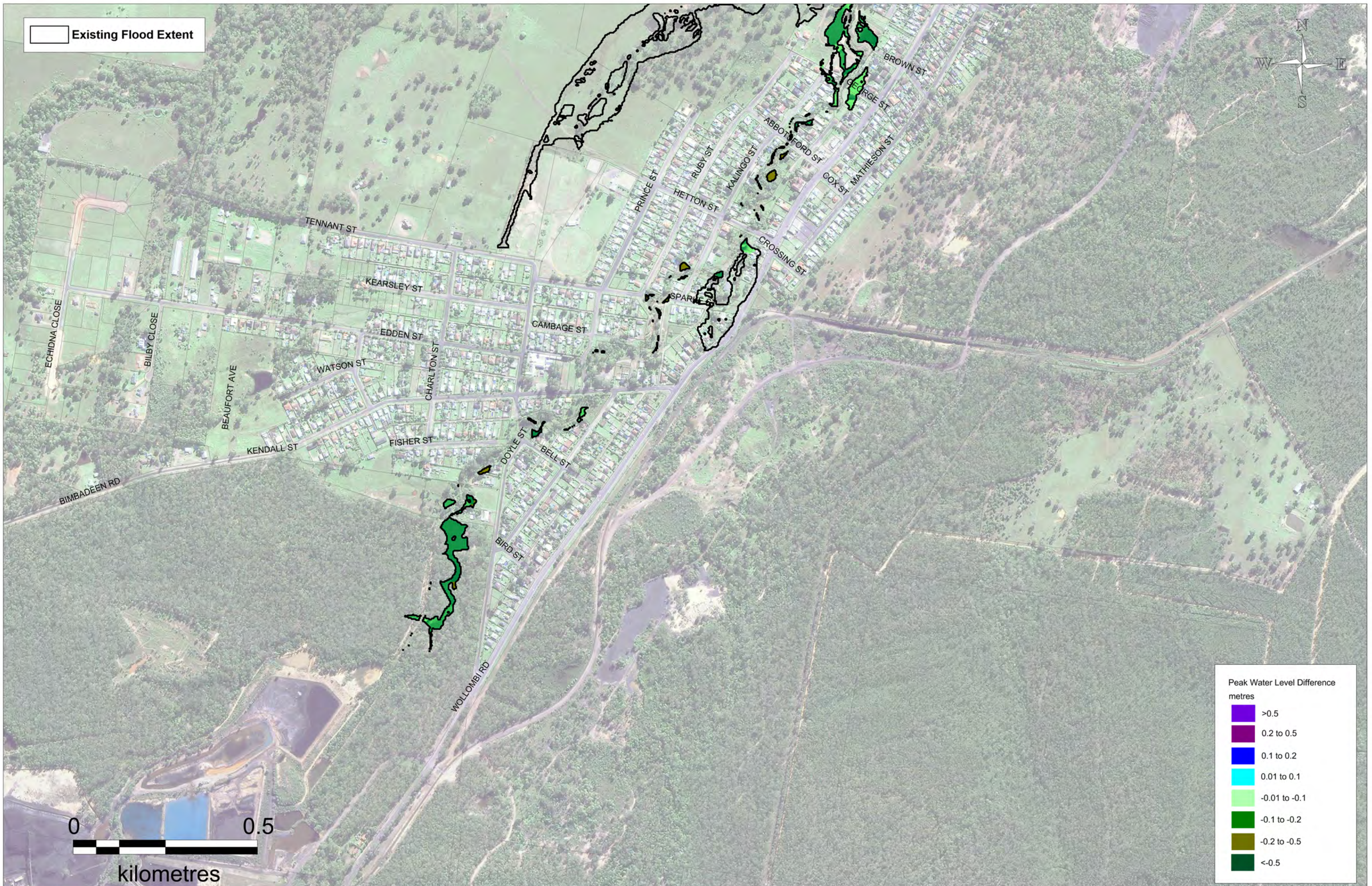
FIGURE 11-42 : APRIL 2015 EVENT - PEAK WATER LEVEL DIFFERENCES FM6 Results Less Existing Results
