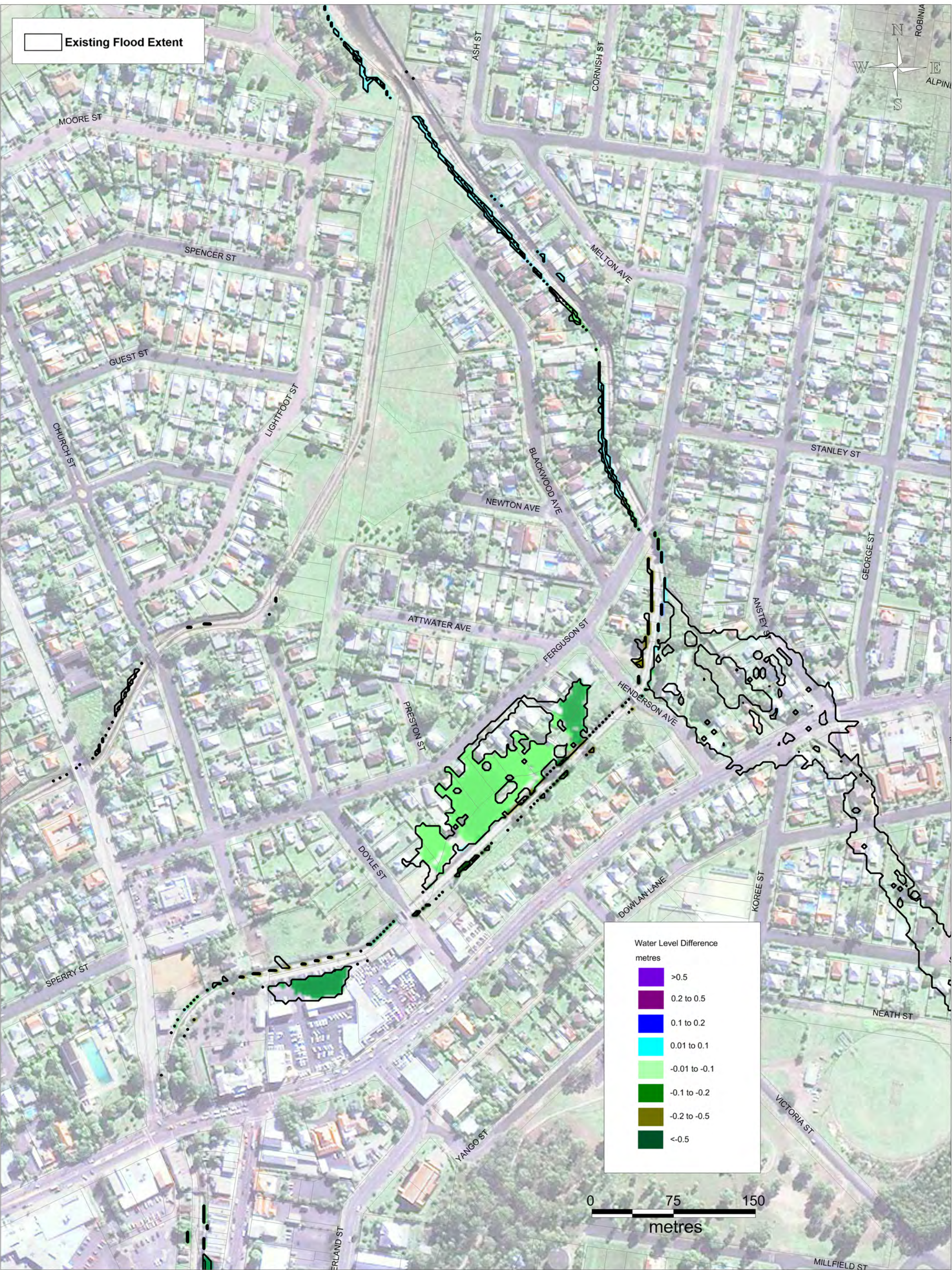
FIGURE 11-20 : APRIL 2015 EVENT - PEAK WATER LEVEL DIFFERENCES FM3 Results Less Existing Results
