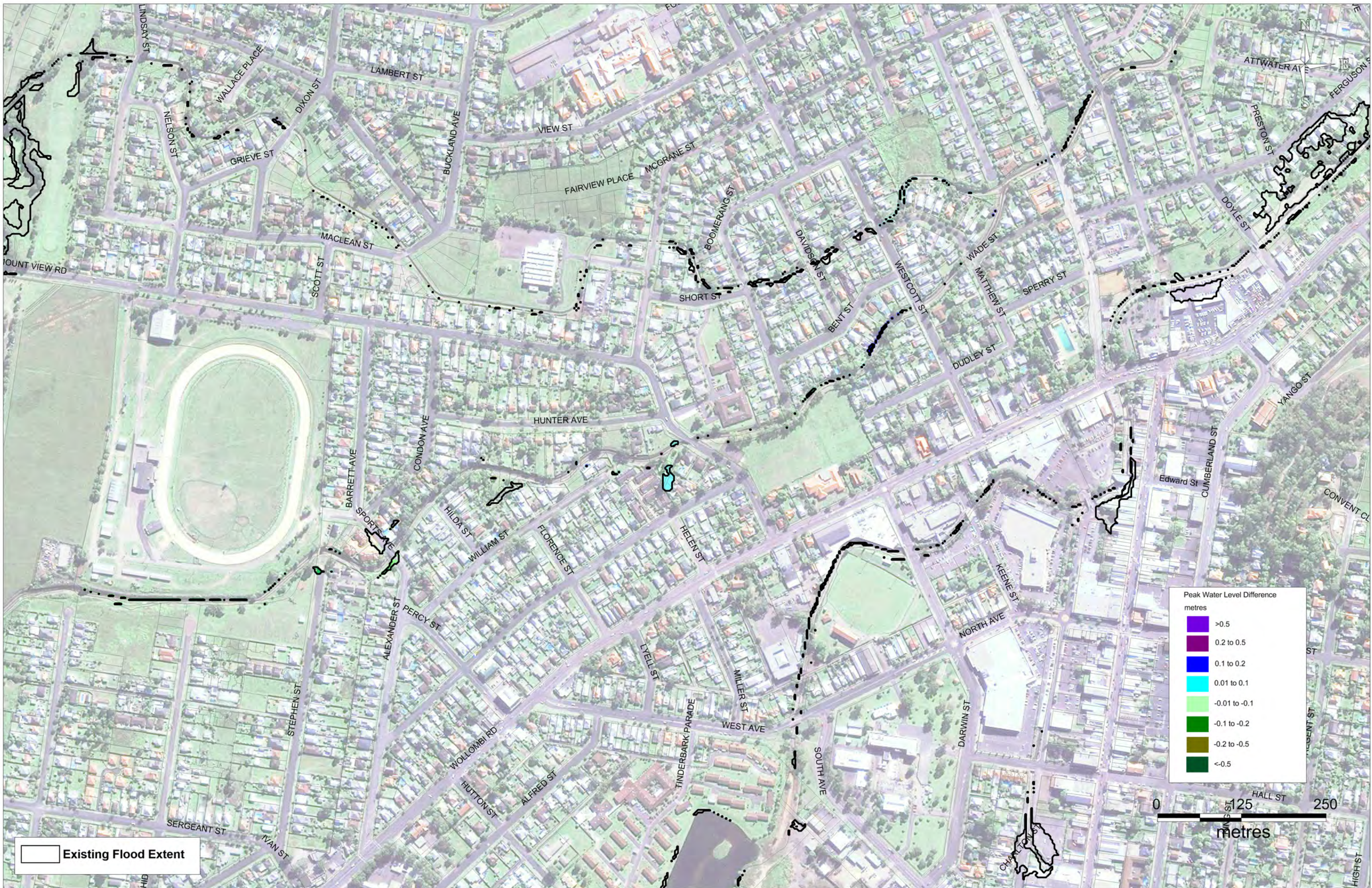
FIGURE 11-13 : APRIL 2015 STORM - PEAK WATER LEVEL DIFFERENCES FM2 Results Less Existing Results
