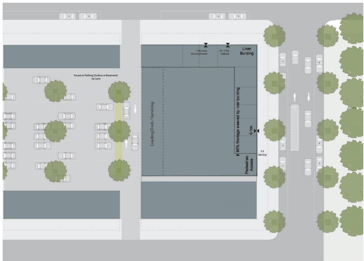
Figure 37: Large format building and liner
