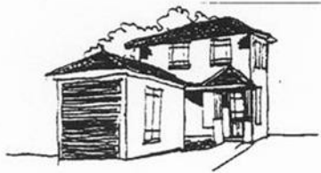
Poor relationship to street - the garage dominates the dwelling when viewed from the street
